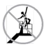
Do not sit, stand, or climb on the platform guard rails. Maintain a firm footing on the platform floor at all times.
