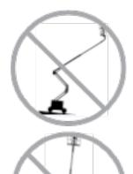
Do not raise or extend the boom unless the machine is on a firm, level surface.
