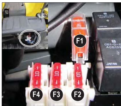
Fig. 10: Fuses (from serial number WNCE0801TPAL0051)
