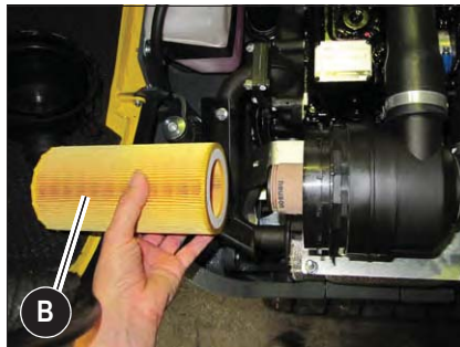
Fig. 24: Removing the outside air filter
