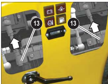
Fig. 54: Ball pins (SAE controls shown)
