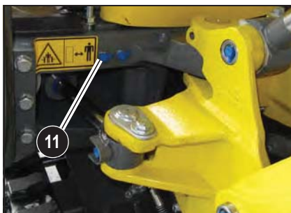
Fig. 49: Lubrication points of ball bearing race
