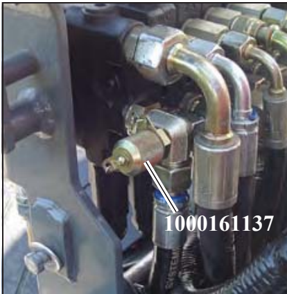
Fig. 29: Secondary pressure limiting valve measurement connection
