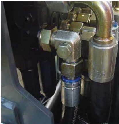
Fig. 28: Plug instead of measurement connection
