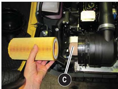
Fig. 25: Inside air filter
