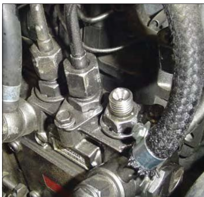
Fig. 8: Opening on fuel pump
