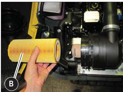
Fig. 22: Removing the outside air filter
