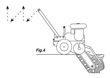
5. Repeat this action until you have finished the job. The wheel lock will aid you in this operation by helping to hold the trencher in position until the next motion is started.
