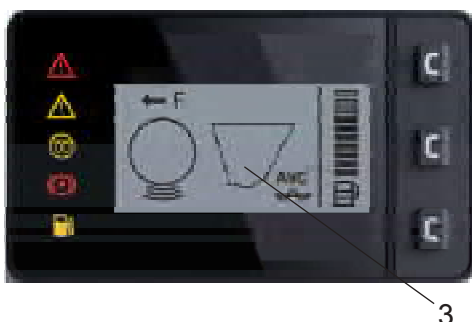
Fig. Working mode, Chip spreader (Off)
