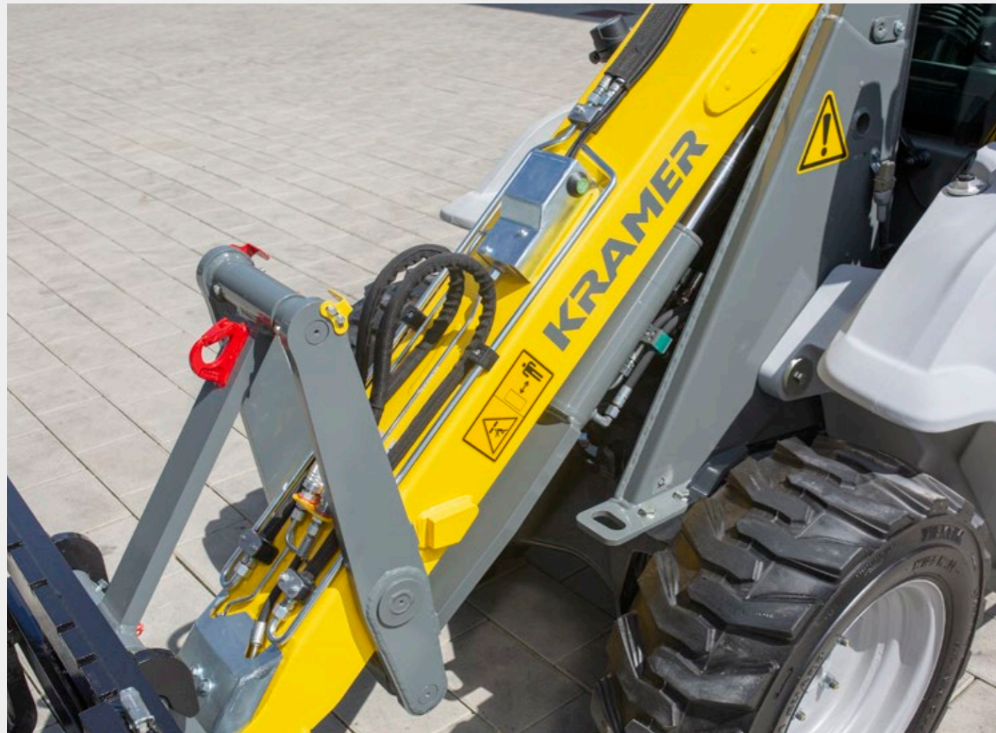
Sturdy loader unit with Z-kinematics, visual position display and optional load hook.
