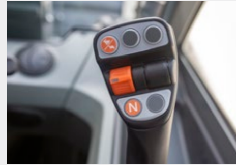
Comfortable joystick: Switch between hare and tortoise directly on the joystick.
