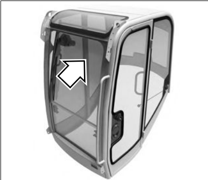
Fig. 73: Opening the front window to a gap
