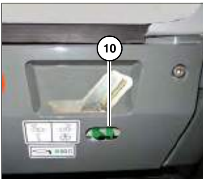
Fig. 241: Lubrication point of ball bearing race
